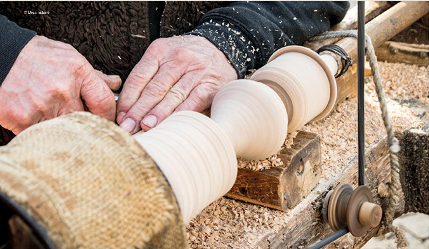
Above: Wooden chair components turned on a pole lathe
